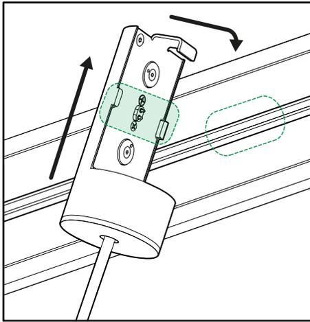
HOOK ON FIXTURE AND ALIGN TABS TO
