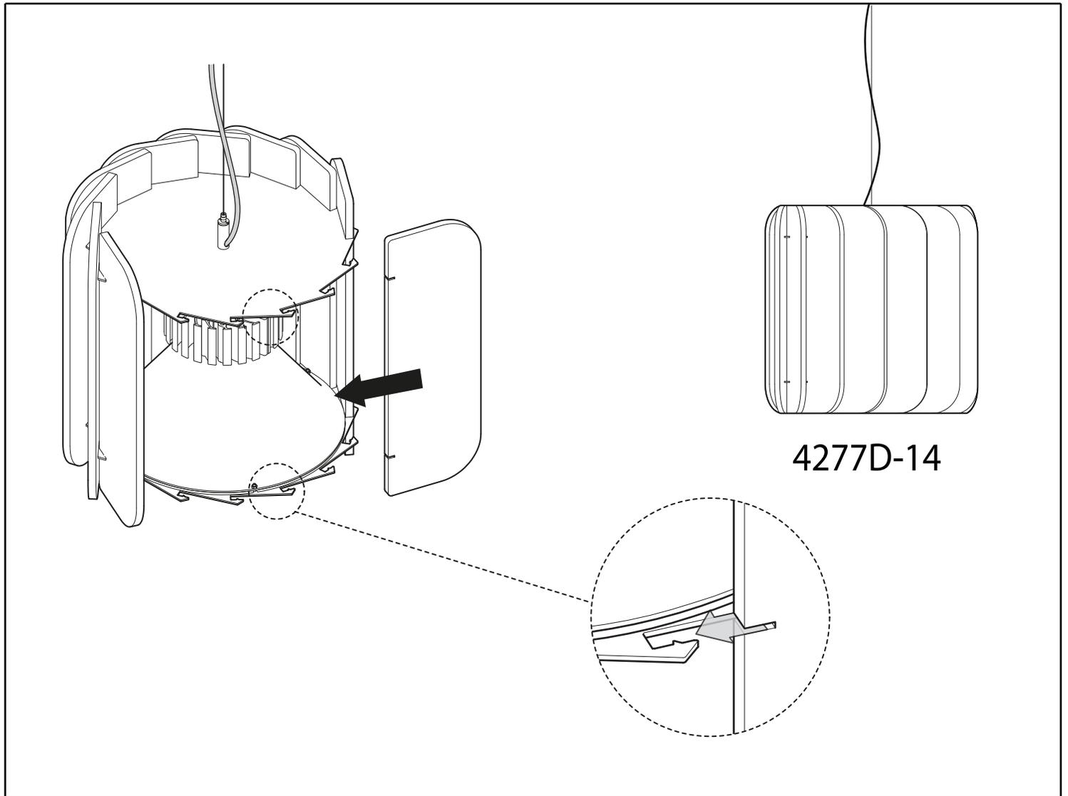
INSERT THE 15 FELT SHADE PANELS BY SLIDING THEM INTO THE TEETH OF THE TWO CORRESPONDING TOOTHED PLATES
