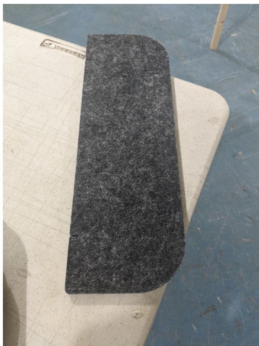
Figure 4 – Individual specimen fin prior to installation to hub
